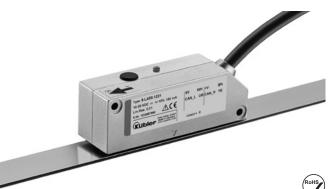
The non-contact absolute magnetic linear measurement system Limes LA50 / BA5 - made up of the sensor head LA50 and of the magnetic band BA5 - reaches a resolution up to 10  $\mu$ m with a maximum distance of 1.5 mm between the sensor and the band.
