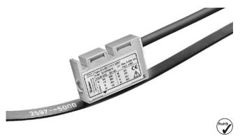
The non-contact incremental magnetic linear measurement system Limes LI50 / B2 - made up of the sensor head LI50 and of the magnetic band B2 - reaches a resolution up to 5 µm with a maximum distance of 2 mm between the sensor and the band.
